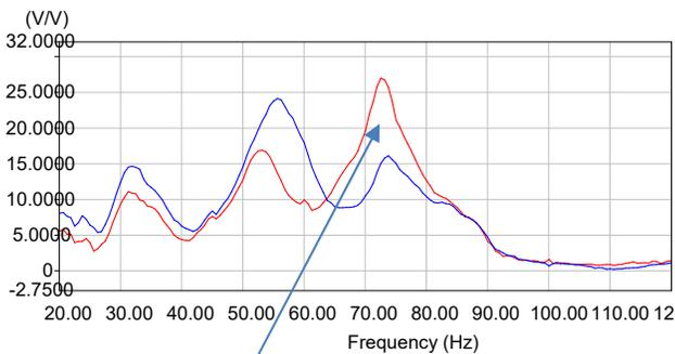
Figure 1 Frequency response function of the cabin, with the cabin entrance closed (red) and open (blue)
