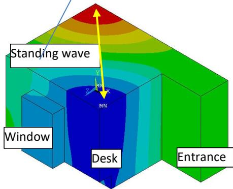
Figure 2 Corner to corner standing wave in the cabin, occurring at around 75 Hz
