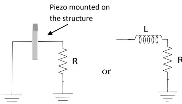
Figure 1 The schematic of a shunted piezo damper
