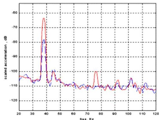
Figure 3 Power spectra of acceleration without (red) and with (blue) shunt piezo damping
