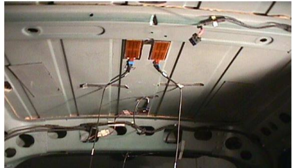
Figure 2 The image of the piezo patches installed on the plate structure
