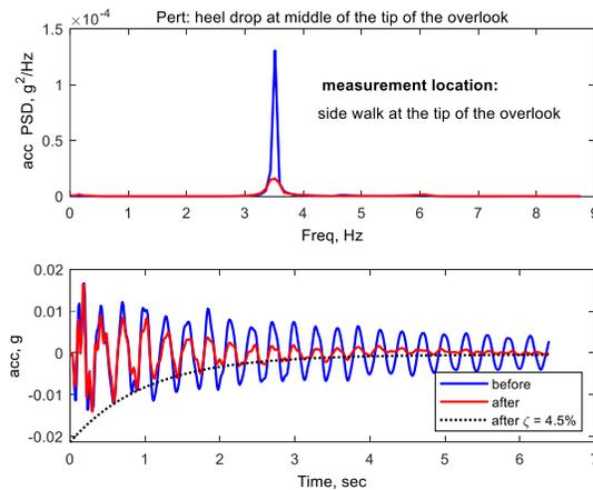
Figure 3 Acceleration PSDs and time responses measured at the tip of the overlook without (blue) and with (red) TMDs with heel drop perturbing the structure at two locations
