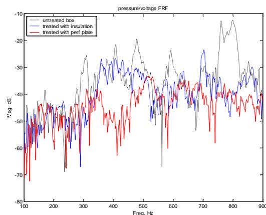
Figure 2 Frequency response functions indicating absorptions with different acoustic
