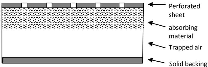
Figure 1 Make-up of perforated acoustic liner
