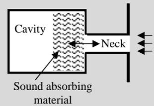
The cavity and neck combination, resemble a spring mass combination, and as such have a *natural frequency* determined by the inertance of the gas in the neck and the compliance of the gas enclosed in the cavity.
