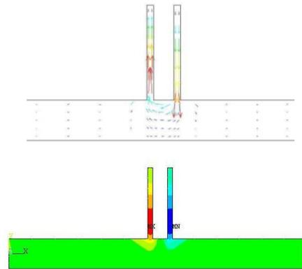
Figure 2 Pressure gradient of two adjacent quarter-wave tubes at the tuning frequency
