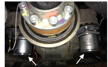
2 PMAs installed on rear sub-frame
