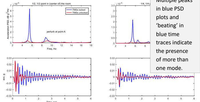
Figure 3 Power spectral densities (PSDs) and time traces of measured acceleration at the center of the floor (the left plots) and the 1/4, 1/4 point (the right plots) in response to heel drop perturbation at the center of the room.
